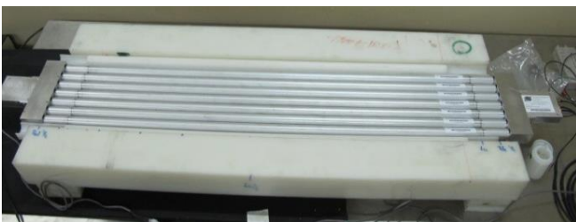
Fig. 2: Boron Coated Straws imaging panel composed of seven detector tubes. The amplifiers 1 and 2 allow getting the ratio of pulse heights that is directly related to the position of the neutron interaction inside the tube.
