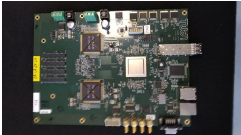
Figure 1.13: Picture of the hodoscope FE card. One FE card is used for the “small” hodoscope whereas four FE cards are used for the “big” hodoscope.
