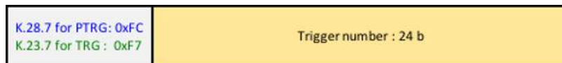
Figure 2.4: Format of the Trigger (TRG) and Pre-Trigger (PTRG) frames, which are composed of 32 bits each.
