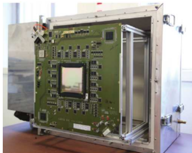
Figure 1.15: (a) Sketch of the silicon scatterer with up to 10 scatter layers mounted on their FE boards with the DSSDs in the centre surrounded by the analog FE electronics (AFEEs) and the Digital Signal Processing (DSPs) performed by FPGAs upstream of the communication channels. (b) Picture of the scatterer detector assembled with one scatter layer mounted on its FE board.
