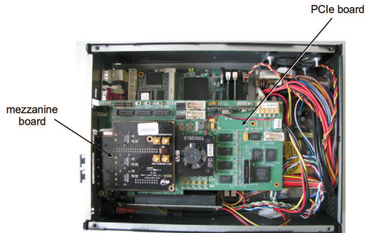
FIGURE 3.29: Picture of the PCI Express board plugged to the acquisition PC with its mezzanine daughter board containing optical transceivers.
